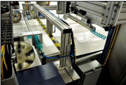
The VMS wheel on a hot air welder marking the Duro-Last deck sheets.
